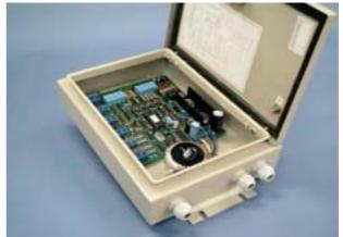
providing full alarm reporting, sensor status monitoring and programmable alarm output control functions from the MEGA-CCTV system. These units can be used individually, or interconnected to configure an alarm network of 16 to 4096 alarm input points, supervised inputs are provided for N.C. alarm contacts for each alarm inputs. The unit requires a 4 core twisted shield data cable which looped to each remote alarm processing unit from the MEGA-CCTV control PC.
